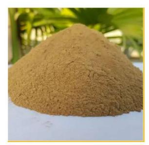
BENTOFOUND is selective high quality and high swelling sodium-based bentonite with high purity and high Thermal Stability. BENTOFOUND is sodium based activated bentonite designed to meet the requirements of modern foundry set up especially high-pressure mouldings lines and deep-drawn castings. BENTOFOUND imparts Low Specific Burn Out Ratio in mouldings sand due to its High Purity, Thermal Durability and high themed stability than Conventional Bentonite.
